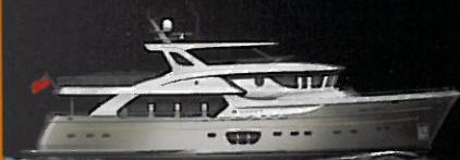
CHINA 92' Selene Ocean Explorer. Guido de Groot Design. Full Displacement w/ bulbous bow. Full ABT Trac hydraulics package.
