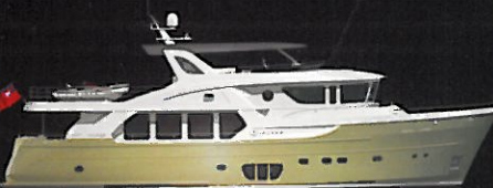
CHINA 75' Selene Ocean Explorer. Guido de Groot Design. Full Displacement w/ bulbous bow. Single or Twin Engine packages. 4 S/R + full crew.
