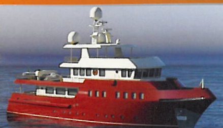
ITALY. 115' Naumachos. Sergio Cutolo design. 7,500nm range. Diesel electric hybrid propulsion. Zero speed stabilization.
